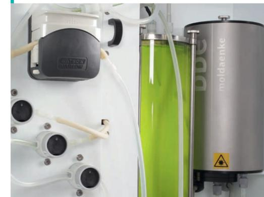
Sample water is mixed with the algae test solution and then analysed.
