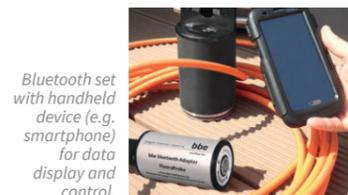
Bluetooth set with handheld device (e.g. smartphone) for data display and control.
